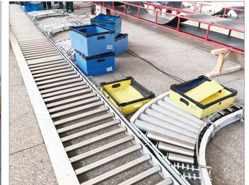
Sorting Interflow Conveyor Line
