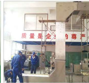
Bucket conveyor for seafood
