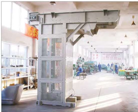
Bucket Hoister Feeder
