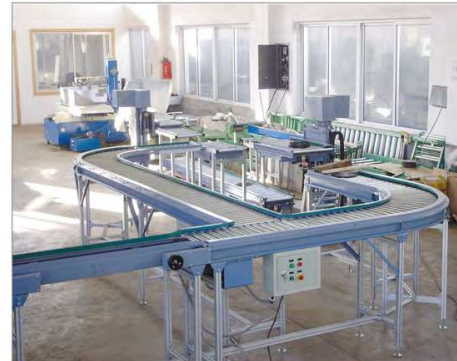
Auto Hoister Interflow Roll Conveyor Line
