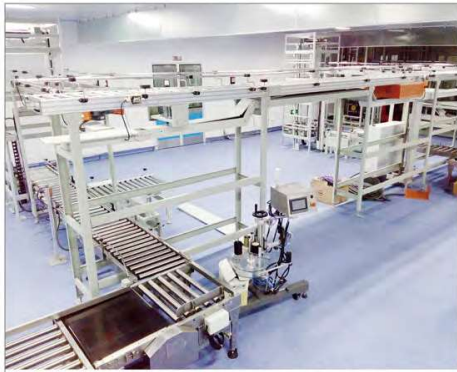
Logistic Conveyor Line For Finished Product
