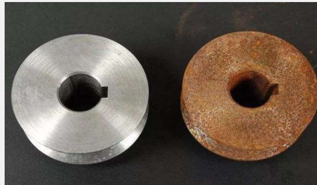
Part Rust Removal
