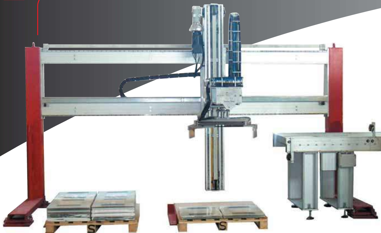
Palletising glass panel wrapped with shrunk film
