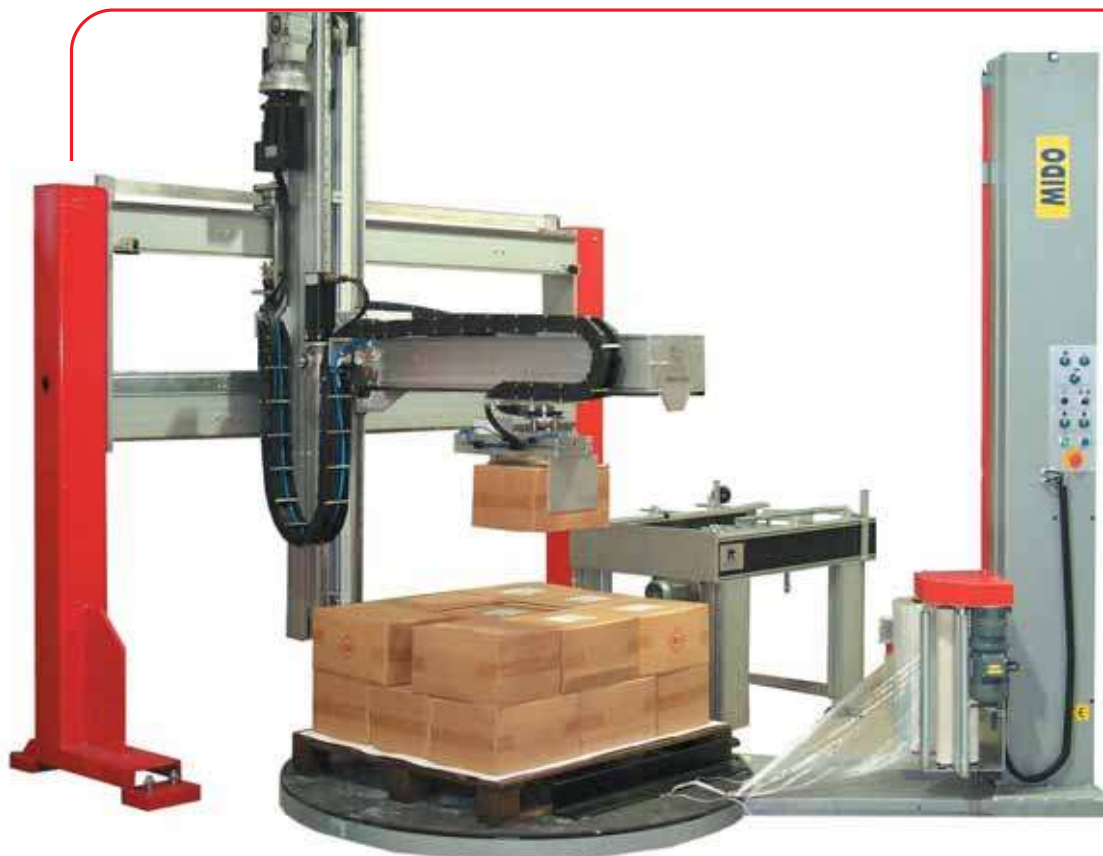
Palletising boxes with film wrapping machine integrated
