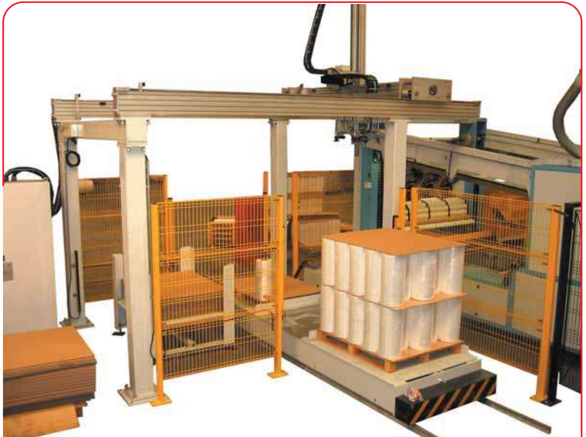
Palletising stretch film rolls with carriage shuttle
