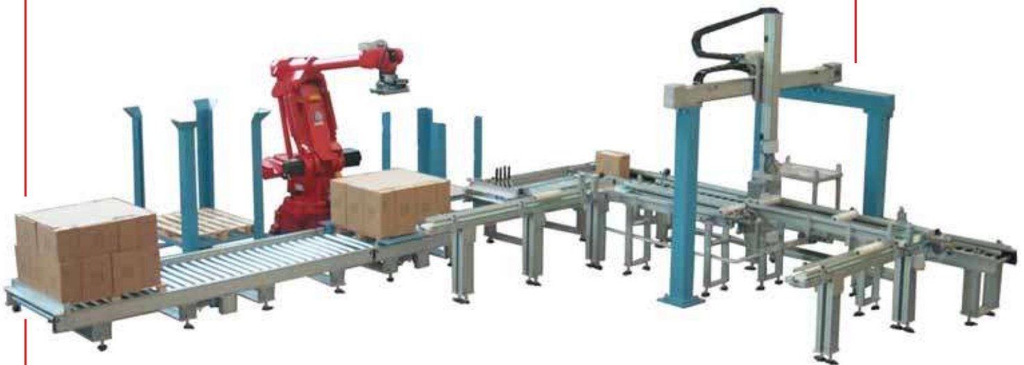
Automatic plant packing film rolls in boxes, labelling and palletising
